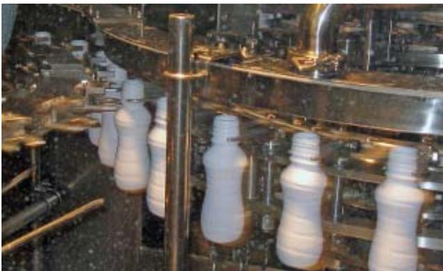
**Bottles enter the enclosure and are picked up by clamps beneath their threads. They are held by clamps throughout the sterilizing/rinsing/filling/capping operations.**
