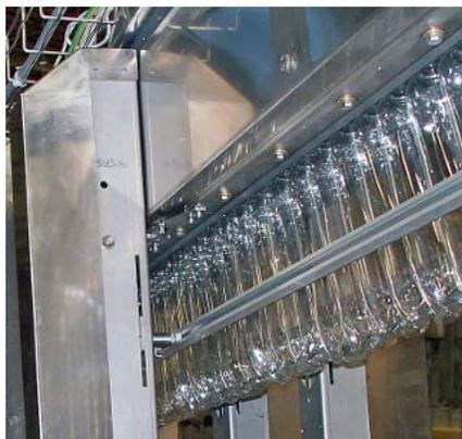
**Bottles are transferred from the mezzanine to the filler by an air conveyor that uses filtered air flowing through a chamber to push them along rails down to the filler.**
