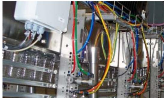
**The air conveyor incorporates a series of sensors and gates that regulate the bottle movement.**
