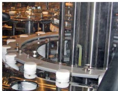
**The 18-head servo-driven capper applies screw caps to the containers. Caps go through a sorter mounted on top of the enclosure and travel through the same hydrogen peroxide sterilizing procedure as the bottles. Constant torque is achieved by a computer-controlled servo motor mounted on each capping head.**
