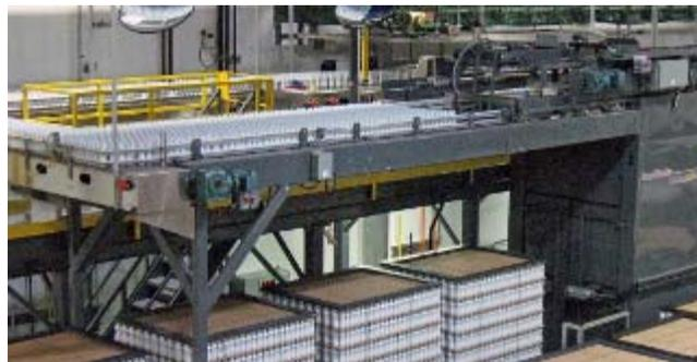
**The bottles are received in bulk and are depalletized onto conveyors on a mezzanine.**
