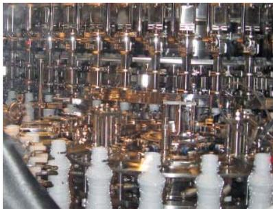
**Bottles are filled on a 81-nozzle net-weight filler. Each empty bottle is weighed after it is in the filler, after which the valve on that nozzle opens and admits product. When the correct weight of product has entered the bottle, the nozzle closes.**
